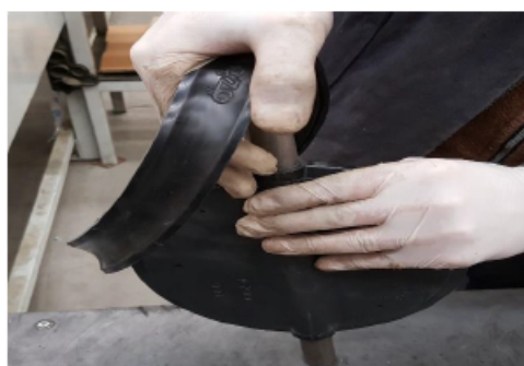
1- Fit the seal on the two sides of disc.
