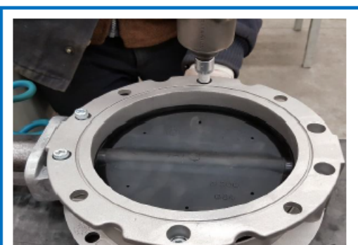
7- Fix bolts and nuts and tighten.
