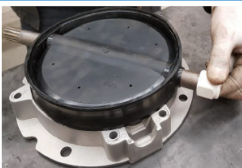
3- Fit bushes on the two sides of disc's shaft.
